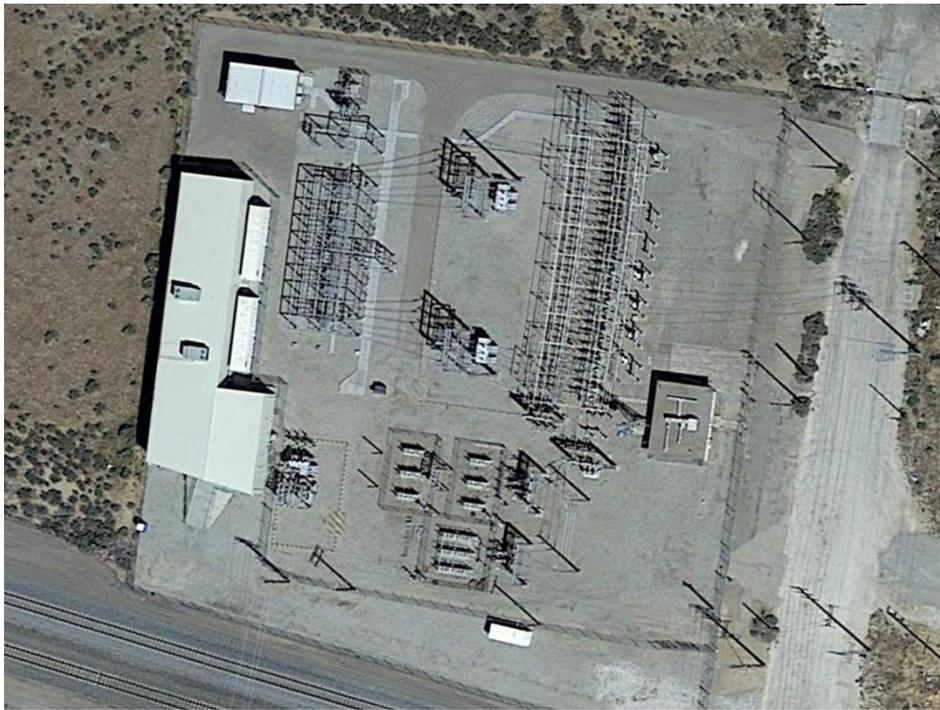
Figure 4. A monolith substation and BESS facility in Tehachapi, California. The BESS provides transmission services, system capacity, and ancillary services. (Source: Google Earth. Appeared in *IEEE Power & Energy Magazine*, vol. 15, no. 5, p. 56, Sept./Oct. 2017.)
