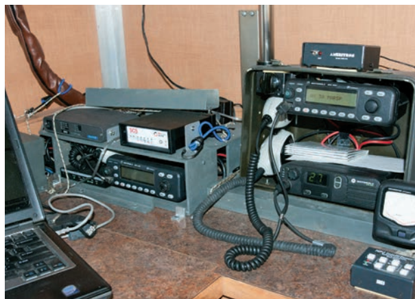
FIGURE 8. Three of the modems are shown. These include the SCS Pactor 3/4 modem, the RapidM RM2 modem for the military M110A mode, and the Kantronics Packet Modem. A modem for Winnor is behind the computer.
