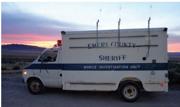
FIGURE 11. The Rover carries VHF mobile communication equipment, six crossed-dipole antennas, and two operators. Here, it is almost ready to start the night ride support, following the pony across Utah's west desert.
