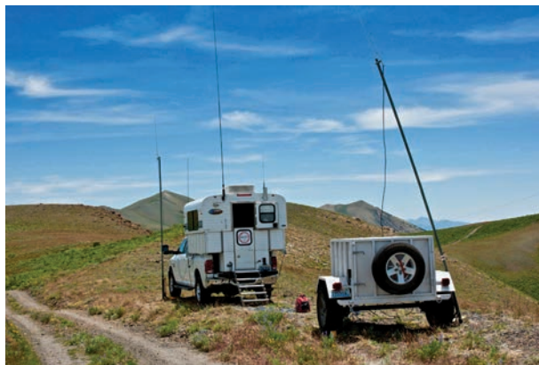
FIGURE 6. This photo shows the 2018 setup at the peak of the Austin Summit. There are two dipoles off to the right of the photo, and the 19-ft whip on the camper shell was used for various HFs through an autotuner.
